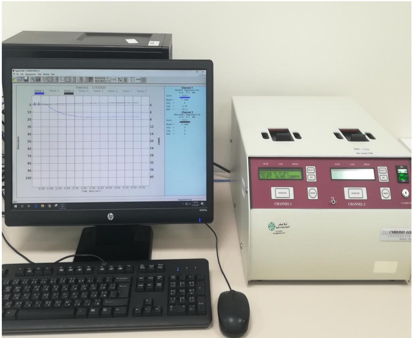
Figure 6: Chrono-log Model 700 aggregometer (Chrono-log cooperation. Havertown, PA, US).
